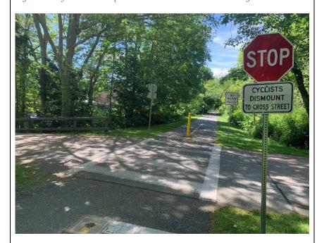
Figure 35: Wayfinding-Oriented Bike Trail Crossing Sign (Road Approach)
