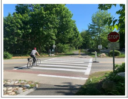
Figure 41: Signage for Eastbound Traffic is Impeded by Foliage
