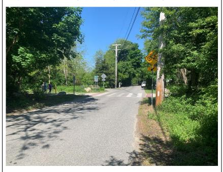
Figure 45: A Wide Crosswalk and Ladder Markings Improve Intersection Visibility
