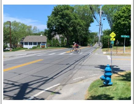
Figure 160: Trail Crossing is STOP Controlled
